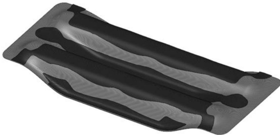
Figure 4-19: CFRP Patch cut of the hybrid side impact beam
