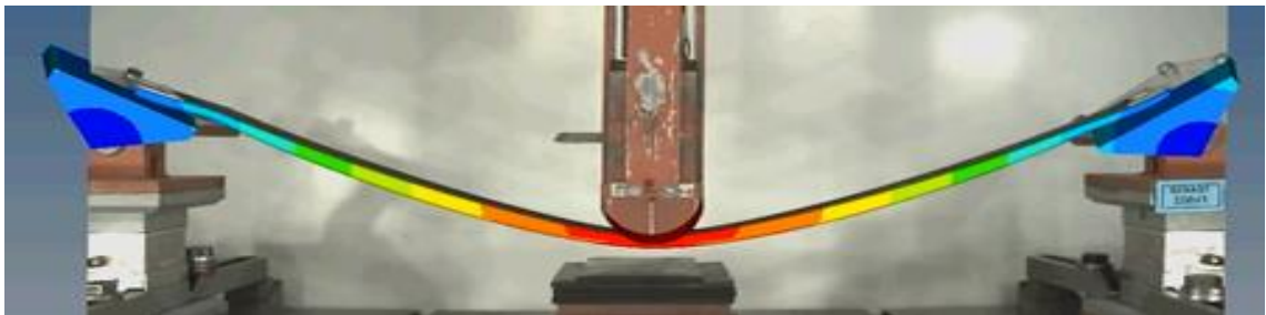
Figure 4-4: Validation of the simulation model compared to the experiment (reference crash-beam)
