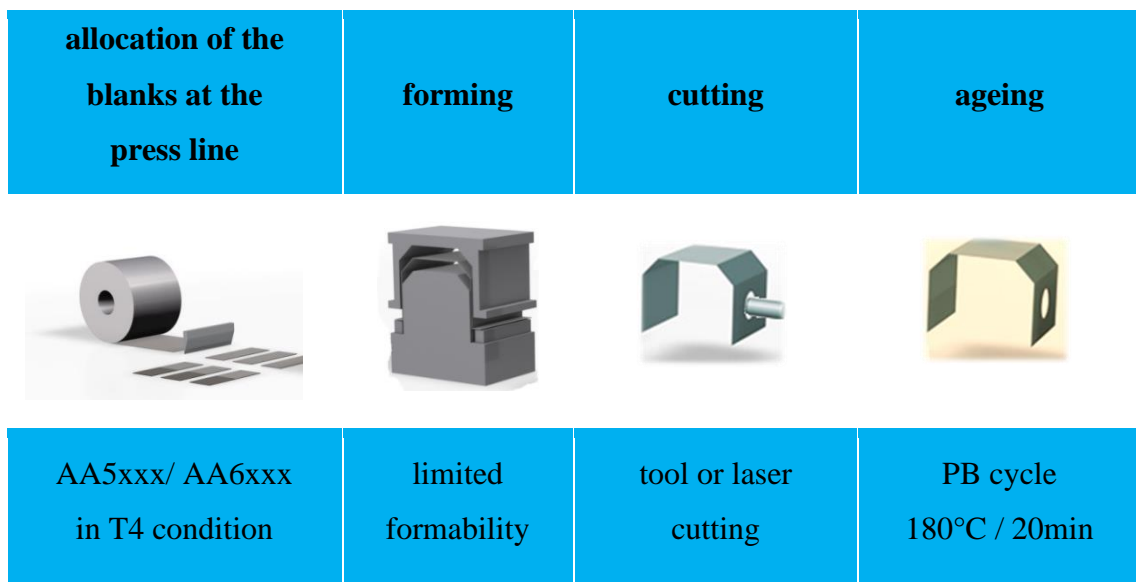
Figure 2-3: Conventional forming process
