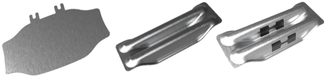
Figure 5-5: Forming of the side impact beam and position of the specimens for the tensile tests
