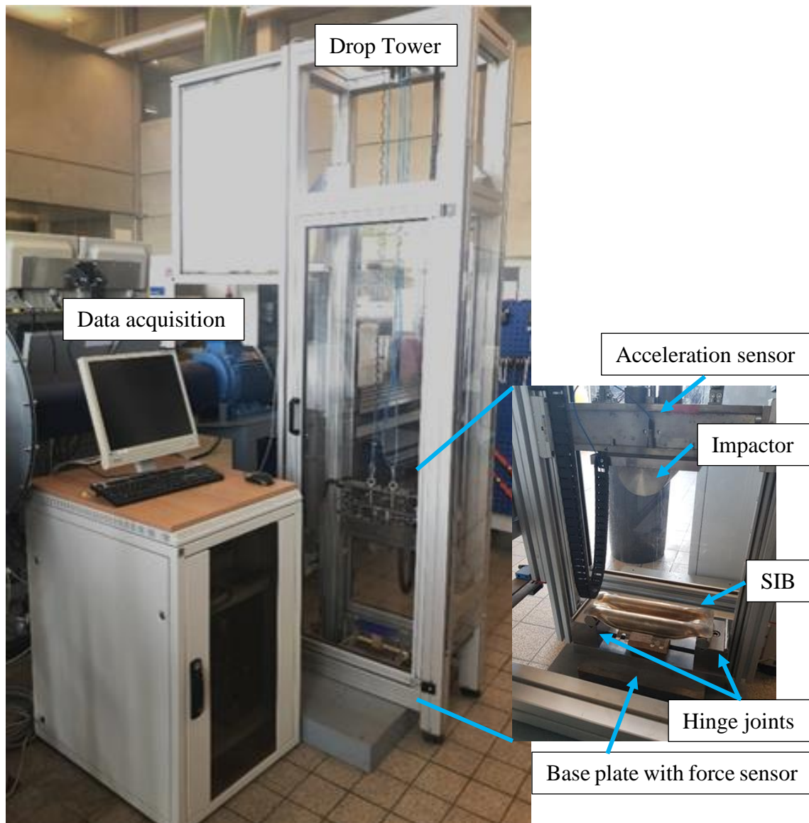
Figure 5-12: Drop-Tower test bench at Aalen university – overview and detail
