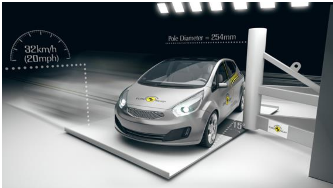
Figure 4-10: Side impact of a car against a pole with a speed of 32 km/h - NCAP test (Euro NCAP 2015)
