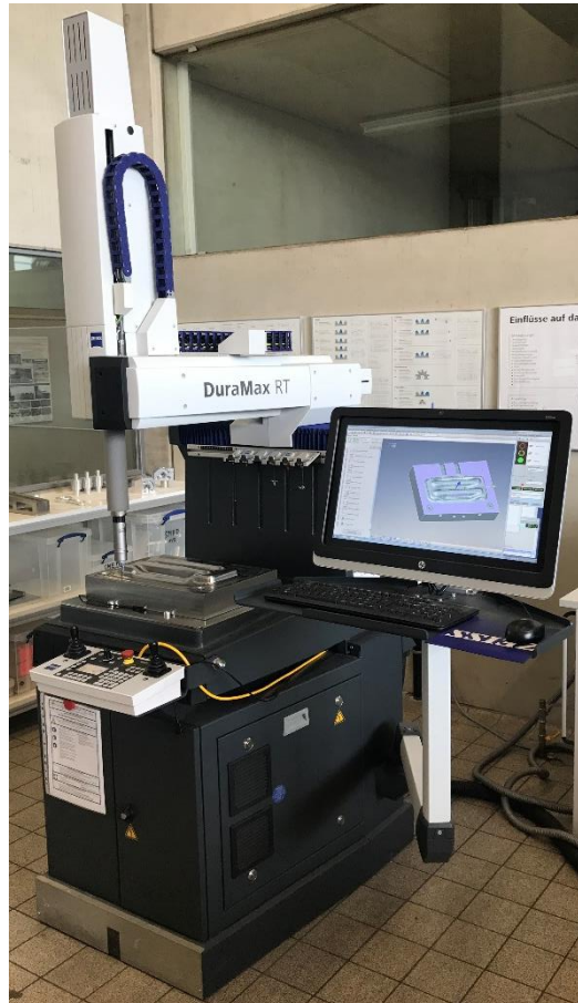
Figure 4-28: Zeiss-DuraMax RT coordinate measuring machine with forming stage
