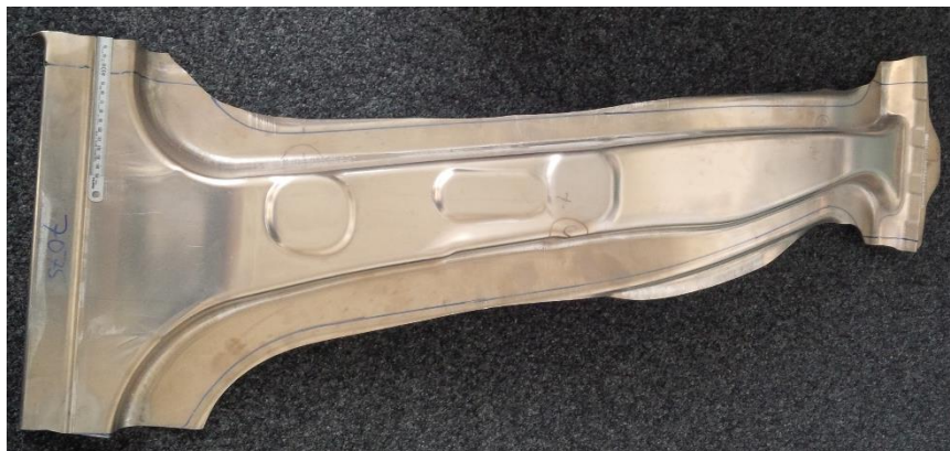
Figure 2-9: W-Temper forming example: B-pillar component
