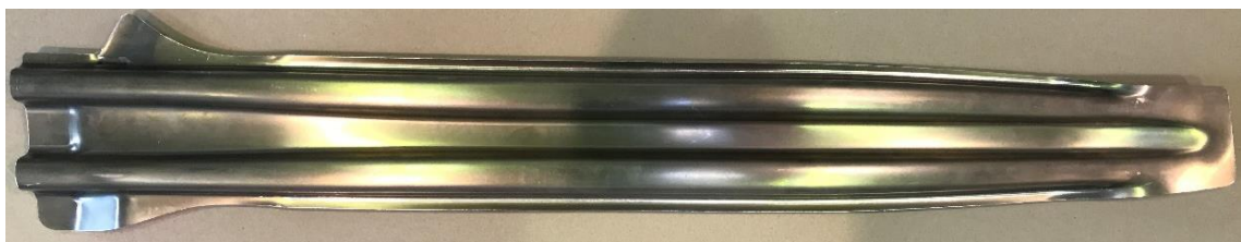
Figure 2-6: Warm-forming example: side impact beam
