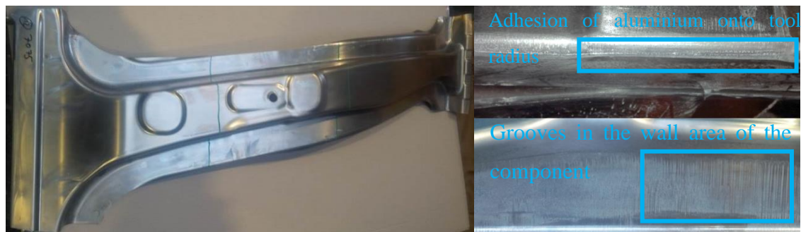
Figure 2-12: Example of the Hotforming process (HFQ®) with a B-pillar component and its problems with adhesion and grooves
